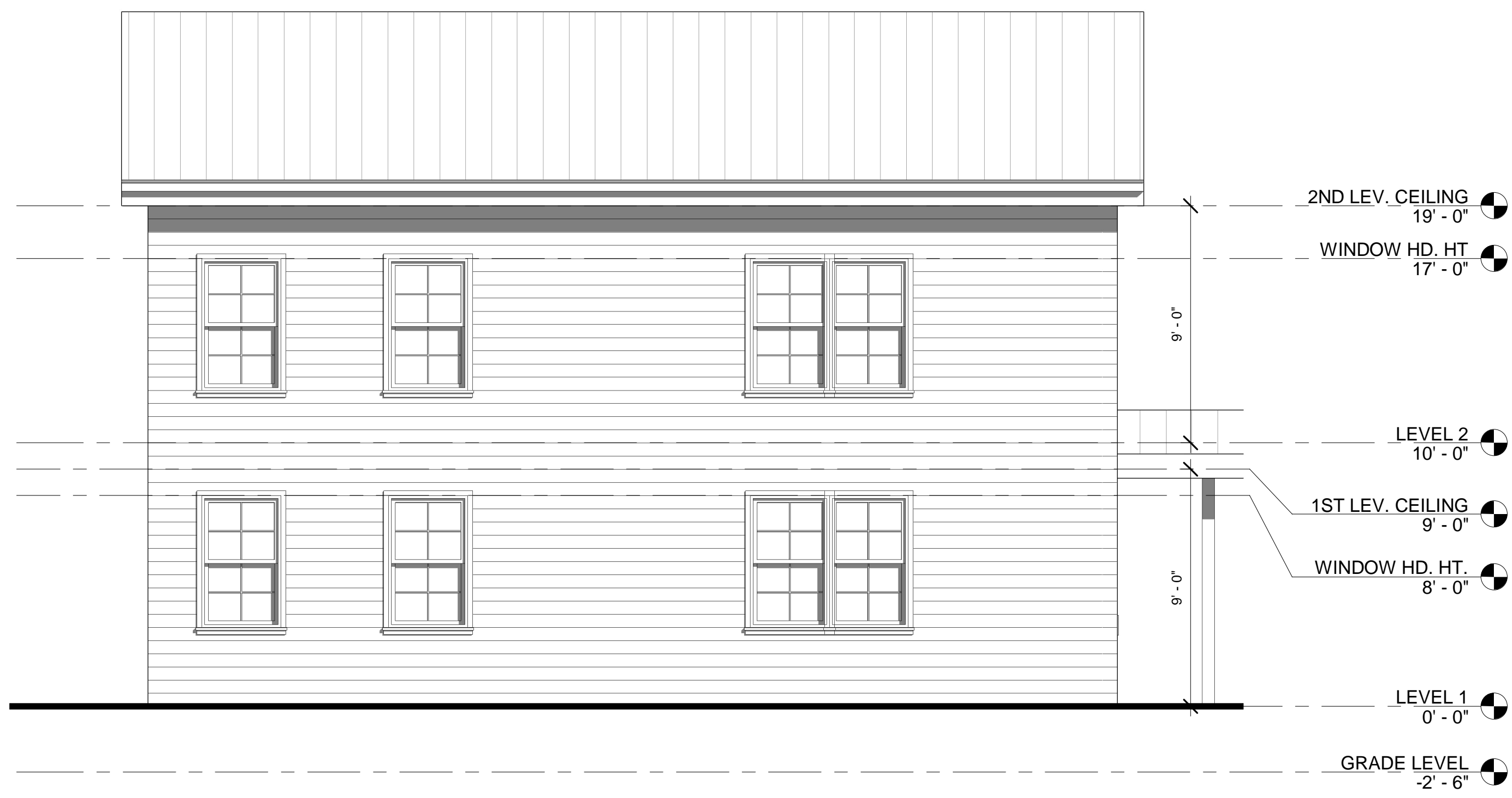
1 EXTERIOR ELEVATION - EAST 1/4" = 1'-0"
